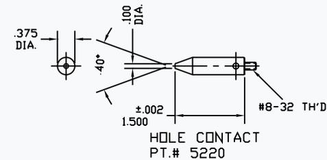
DIAMETER, LENGTH AND DEPTH CONTACT
